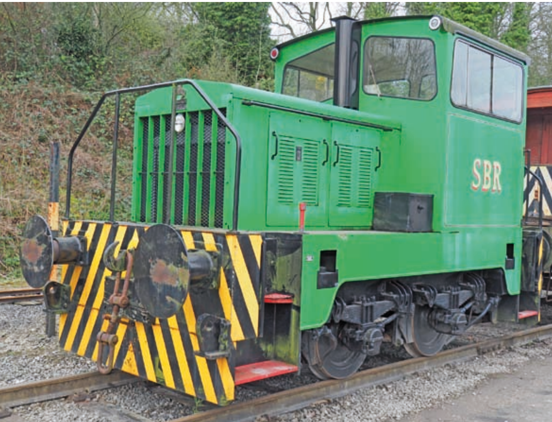
Our New Yard Diesel Shunter. converted from a Sentinel Vertical Boiler steam engine by Thomas Hill of Kilnhust for the CEGB. Was preserved at Statfold Barn Railway.
